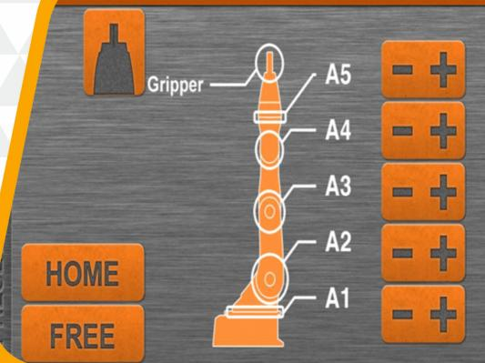
Handling the YouBot via wired mechanism is hectic in complicated tasks. Android application enables to control the YouBot connected over the Wi-Fi or Bluetooth. The Android based application is used to remotely control the KUKA YouBot via an Android smart-phone/Tablet. The control the KUKA YouBot BASE and ARM by selecting different controller modes. It uses the BlueZ library and a Blue-tooth interface. Different other programs will be integrated into the Android APP.
